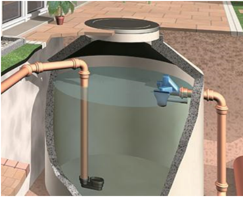
Schematic Illustration of Calming Inlet & Overflow
